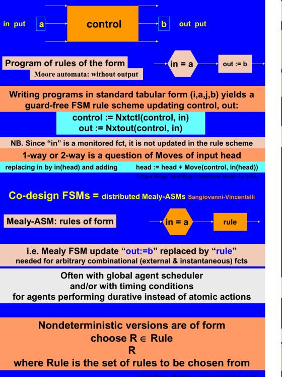
Specializing Mealy to Stream Processing Ctl State ASMs (Janneck 2000)
