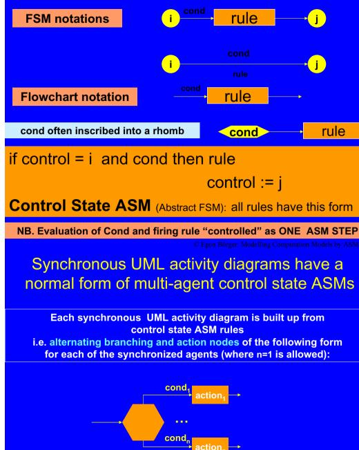
Therefore every synchronous UML activity diagram can be viewed as a synchronous multi-agent ASM whose agents are control state ASMs with rules representing alternating branching and action nodes
